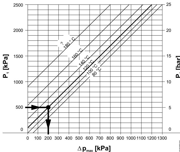
$\Delta p_{\max}$  = Differential pressure at a nearly closed valve to largely avoid cavitation
