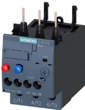
Overload relay 17...22 A Thermal For motor protection Size S0, Class 10 Contactor mounting Main circuit: Screw Auxiliary circuit: Screw Manual-Automatic-Reset
