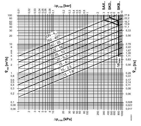
Δp<sub>max</sub> = Maximum permissible differential pressure across the valve (mixing: port A - AB, B - AB), valid for the entire actuating range of the motorized valve
