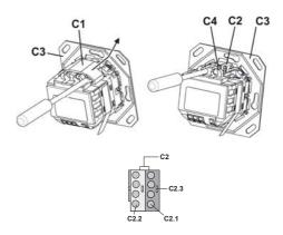
figure 4: Slipping off/on bus connection blocks
