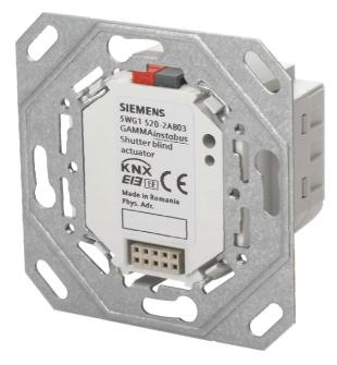
The UP 520/03 shutter / blind actuator with mounting frame is a KNX device with one relay output and a Bus Transceiver Interface (BTI). The device is installed in a flush-mount wall box (60 mm Ø, depth 60 mm). The bus is connected via a bus terminal block. The actuator electronics are supplied via the bus voltage.
