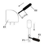
figure 6: Connecting/disconnecting mains and load circuit
