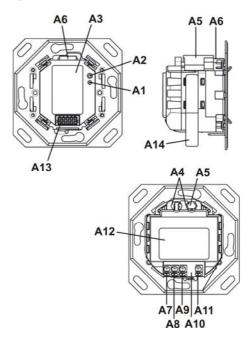
figure 2: Location and Function of the Display and Operating Elements
