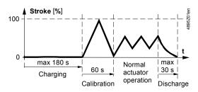
On completion of the charging process and self-calibration (see below), the "Open" and "Close" travel are proportional to the DC 0...10 V control signal.
