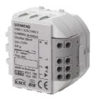
The RS 520/23 shutter / blind actuator is a KNX device with one relay output. The device is installed in an AP 118 Control Module Box or an AP 641 Room Control Box. The bus is connected via a bus terminal block. The actuator electronics are supplied via the bus voltage.
