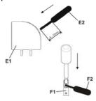
figure 6: Connecting/disconnecting mains and load circuit
