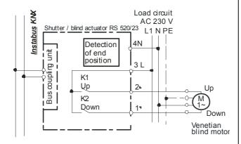
figure 1: Example of operation
