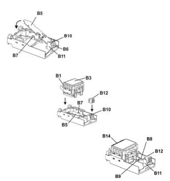
figure 2: Mounting of a RS module
