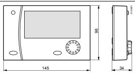
Drilling template for front mounting
