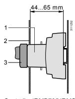
Controller/RMB795/RMS705 complete with attached operator unit is mounted inside the control panel; the operating elements are accessed through a cutout in the control panel door (external operation).
