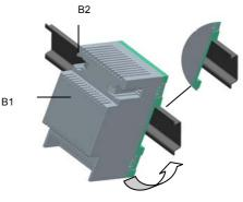
Figure 3. Mounting the device
