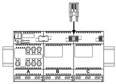
Figure 5. Connecting a switching actuator submodule
