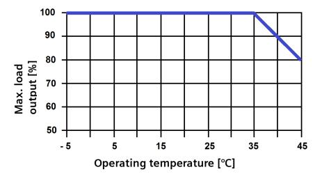
Fig. 7 max. load output derating diagram
