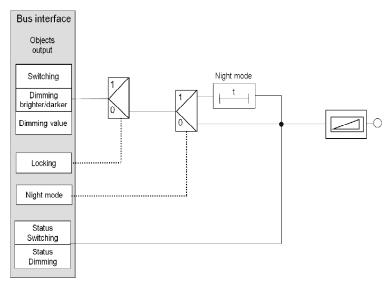
Fig. 3 Schematic design of a dimming actuator channel
