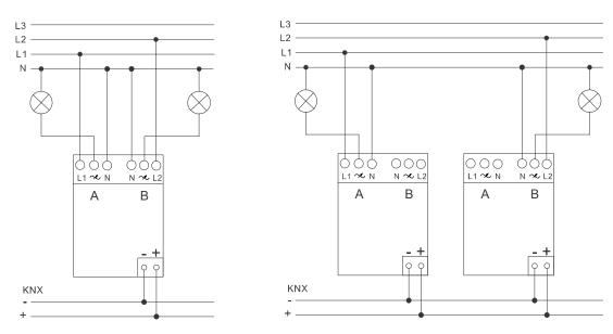
Fig. 1 Schematic applications
