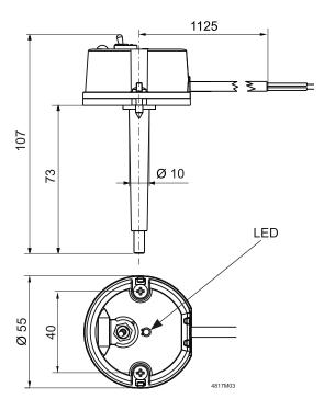
Actuators for fire and smoke protection dampers GGA126.1E/.., GGA326.1E/..
