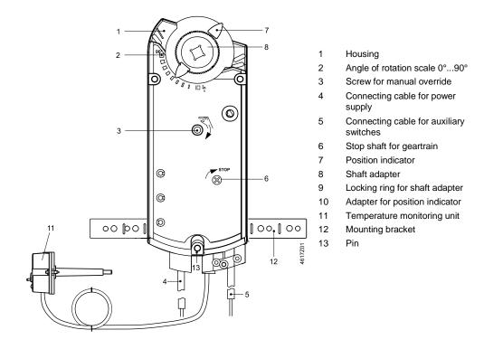
Arrangement for shaft adapters
