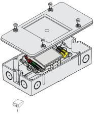
Installation in range with enclosed mounting feet at top hat rail TS35
