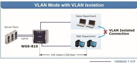
In the **Extend operation mode**, the WGS-810 operate on a per-port basis at 10Mbps duplex operation but over a distance of up to 250 meters overcoming the 100m limit on Ethernet UTP cable. It also supports VLAN isolation to isolate ports so as to prevent broadcast storm and defend DHCP spoofing in the extend operation mode.
