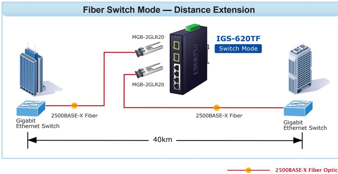
**Adjustable 6-Port Switch Mode or 4 + 2 Fiber Redundant Mode**
